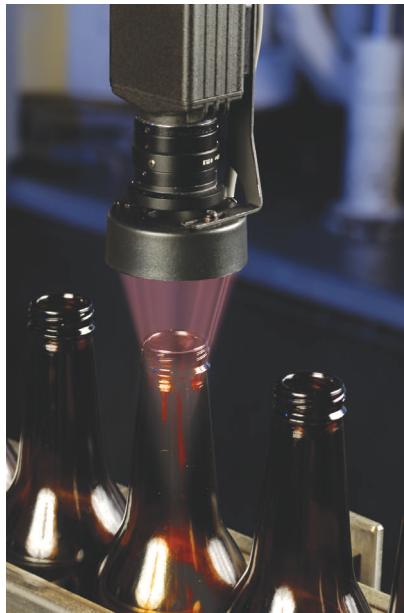
FIGURE 2. A ring light attached to a camera illuminates the bottom of a bottle so an inspection system can check for cracks or other defects. Courtesy of Advanced Illumination.
